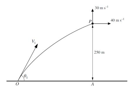
A particle P is projected with speed  $V_1 \,\mathrm{m\,s^{-1}}$  at an angle of elevation  $\theta_1$  from a point O on horizontal ground. When P is vertically above a point A on the ground its height is 250 m and its velocity components are  $40 \,\mathrm{m\,s^{-1}}$  horizontally and  $30 \,\mathrm{m\,s^{-1}}$  vertically upwards (see diagram).
