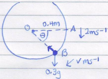
(a) By the principle of conservation of energy, the total energy at A is equal to the total energy at B.
