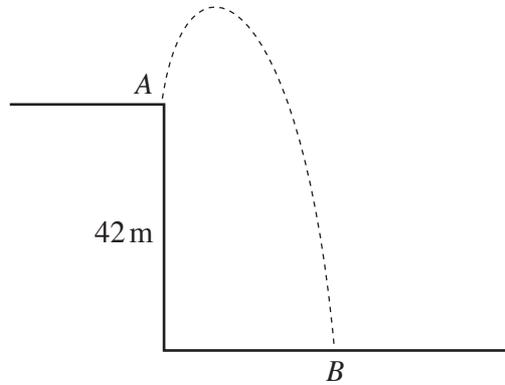
The horizontal and vertical components of the stone's initial velocity are  $4.5 \text{ ms}^{-1}$  and  $22.4 \text{ ms}^{-1}$  respectively.
