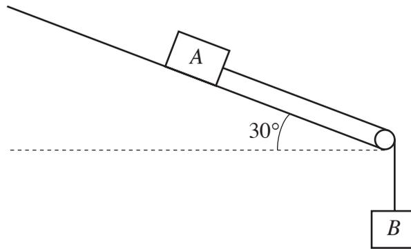
The system is released from rest. Find the magnitude of the acceleration of object A and the tension in the string. [7]
