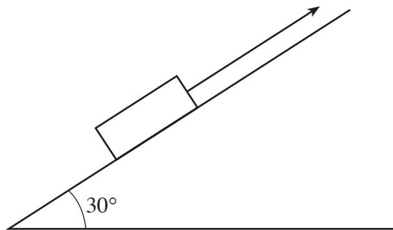
When the tension of the rope is  $12 \text{ N}$ , the sledge slides **down** the hill. Calculate the magnitude of the acceleration of the sledge, giving your answer correct to one decimal place. [6]
