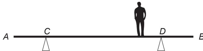
The diagram shows a uniform plank  $AB$ , of mass 20 kg and length 2.4 m, supported in horizontal equilibrium by two pivots, one at  $C$  and one at  $D$ . The distance  $AC$  and the distance  $DB$  are both 0.5 m. A person of mass 40 kg stands at a point which is 0.6 m from  $B$ .
