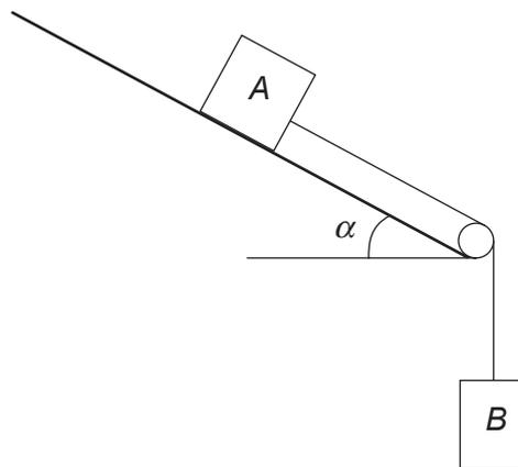
Initially, the objects are held at rest with the string just taut. The objects are then released so that  $A$  slides down the plane.
