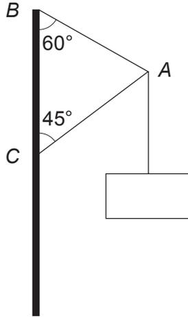
Calculate the tension in  $AB$  and the thrust in  $AC$ .
