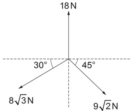
Find the magnitude of the resultant force and determine the angle it makes with the  $18\text{ N}$  force. [8]
