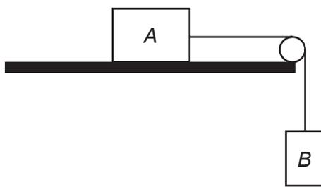
Initially,  $B$  is supported so that the objects are at rest with the string just taut. Object  $B$  is then released.
